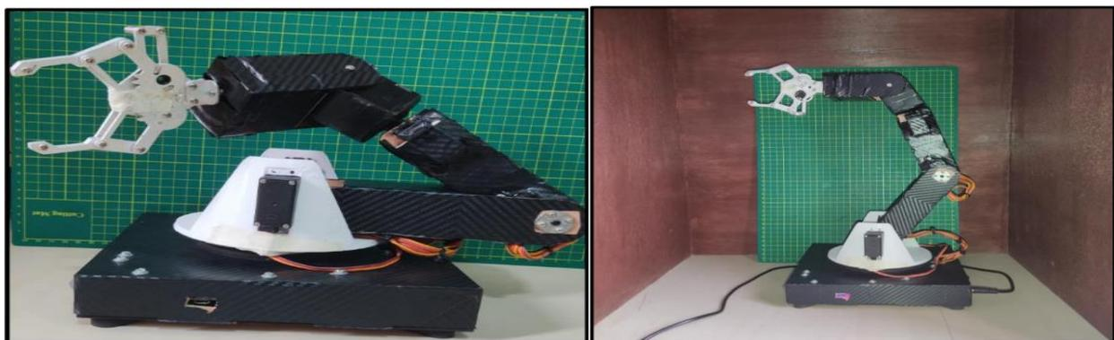
In the current design, configuration and parts used, the arm has a maximum load capacity of 200 gm when fully extended. The cost of the entire project was also minimized and kept under ₹10,000.
